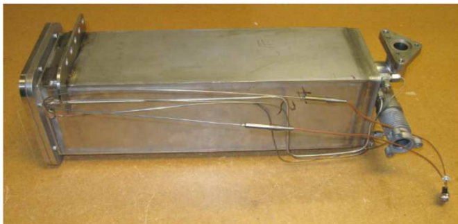
hot reformat desulfurizer
